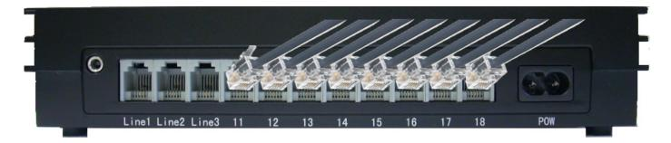
Finally: Connect the power cable to the Mini-PABX (Marked "POW" for Power) on the right side of the image above and then to the power-outlet. After checking that all the above is correct, switch on the power to the Mini-PABX.
